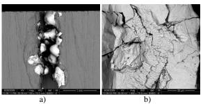
Fig. 3. The overview of the remelted zone of sample P3: a) Conglomerates (100X), b) Carbide's fragmentation (1600x)
