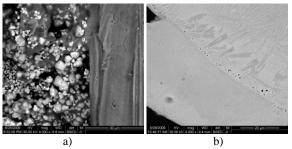
Fig. 2. The carbide distribution for sample P2: a) Carbide's distribution (4000X), b) Cellular growth appearance into the carbide rich particle during solidification (4000X)
