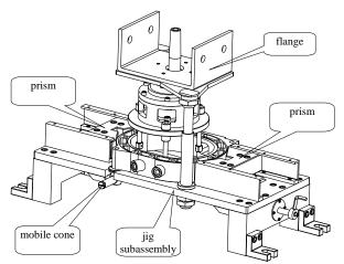
Fig. 5. Device assembly
