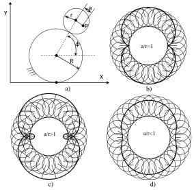
Fig. 2.Epicycloid parameters and different particular cases
