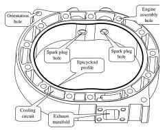
Fig. 1.Wankel housing with epicycloid inside profile
