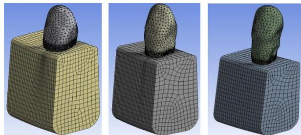
Fig.1 Geometrical models of the three situations taken into this study (normal bone height, 3 mm bone loss, 6 mm bone loss).
