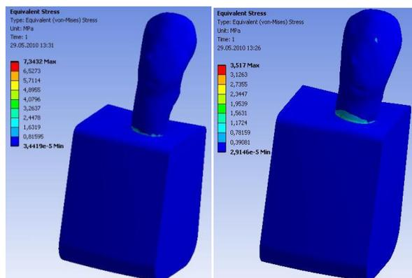
Fig. 3. Stress distribution of the model with 6 and 3 mm bone loss.
