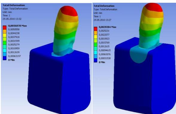
Fig.4. Initial displacement in a canine with 6 and 3 mm bone loss.
