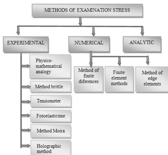
Fig. 1. Method for measuring the stress
