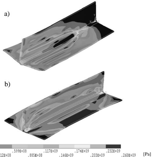
Fig. 4. Misses stresses a) at the time of 30 s b) after cooling
