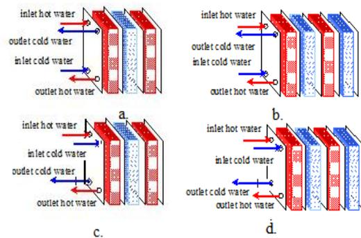
Fig.1. Functional schemes of plate heat exchangers: a. 4 plates counter-flow; b. 5 plates counter-flow; c. 4 plates parallel-flow; d. 5 plates parallel-flow
