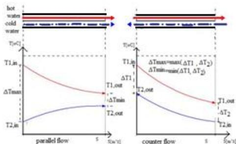
Fig.3. The temperatures distributions in heat exchanger
