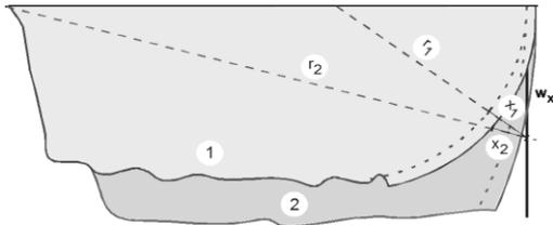
Fig. 2. Geometrical dependence of the factors of seam joining with two different radii of the curvature of the work pieces
