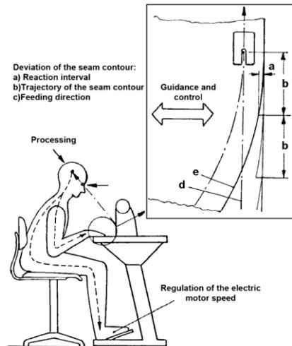
Fig. 1. Man-machine system as a control circuit
