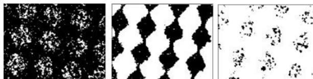
Fig. 4. Images of the 50% coverage values processed in solution with 0.2 moldm -3 , 0.5 moldm -3 and 1.0 moldm -3 conc
