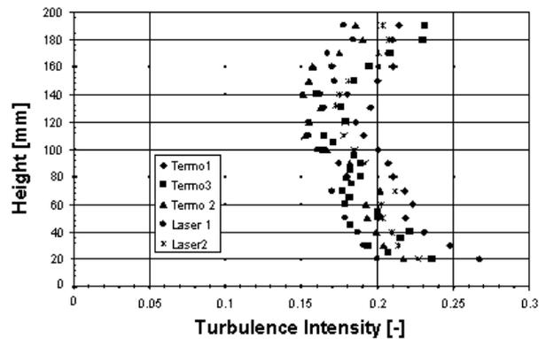
Fig. 4. Vertical distribution of the turbulent intensity in the test section of the wind tunnel with discontinuity at  $x = 1280$  mm distance downstream the contraction cone
