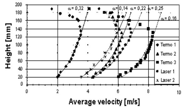
Fig. 3. Mean velocity profile in the test section of the wind tunnel with discontinuity at  $x = 1280$  mm distance downstream the contraction cone
