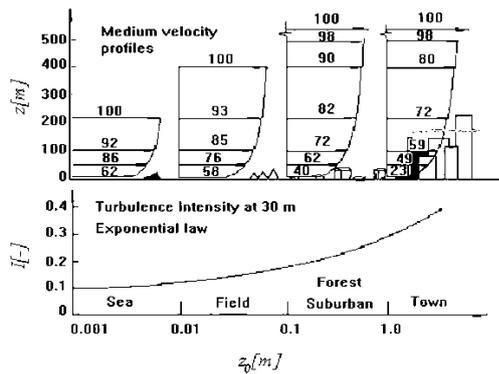
Fig. 1. Mean velocity profiles based on power law and turbulence intensity in the atmospheric boundary layer for different land roughness types
