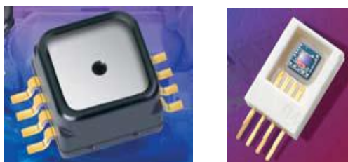
Fig. 1. MEMS sensor of pressure for industrial and medical utilizing
