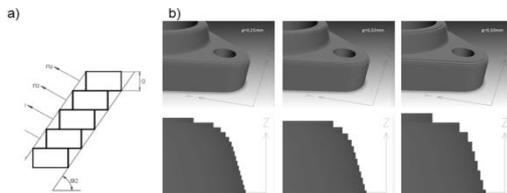
Fig. 5. The essence of staircase error (a) and impact of disposed layer thickness on the error value (b)
