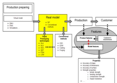
Fig. 1. Features and methods of producing physical models
