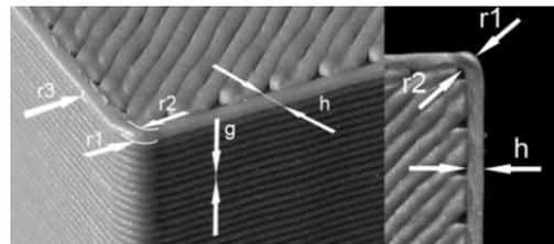
Fig. 8. Illustration of internal error; h - width of single material thread, r1 and r2 - external and internal radius of real model corner, g - layer thickness, r3 - radius of material thread rounding.
