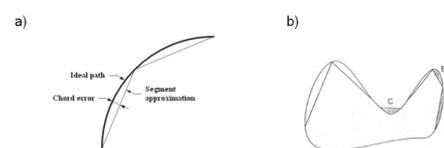
Fig. 3. Error of conversion to STL format; chordal error (a), model error (b)
