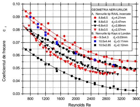
Fig.5. Friction coefficient variation for sinuous fins compared to Kays and London type fins
