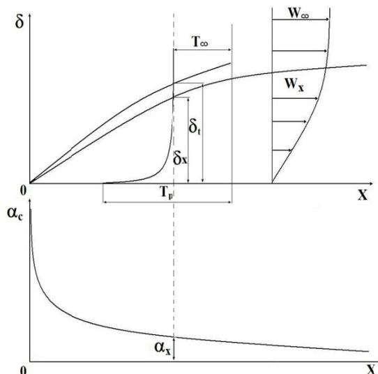
Fig. 1. Hydraulic limit layer at the entry on a plane surface
