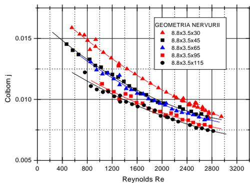
Fig.3. Colborn criteria variation for sinuous fins with 3,5 mm pitch
