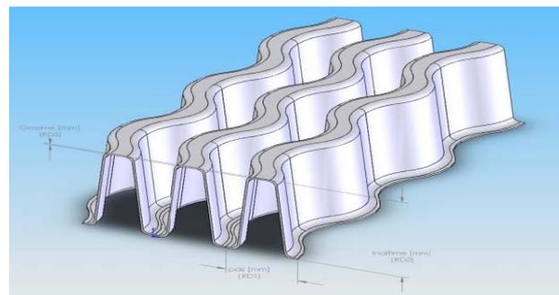
Fig. 3. Sinuous fin used for tested heat exchangers
