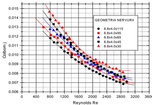
Fig.4. Colborn criteria variation for sinuous fins with 4,0 mm pitch
