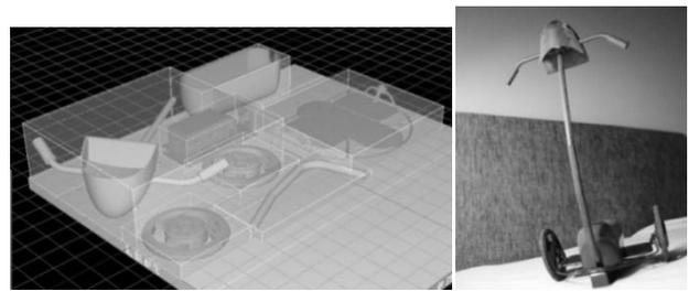
Fig. 5. Best fabrication orientation of the scooter parts on the build platform, Case study "C" (left) and the scaled prototype of the self-balancing scooter (right)
