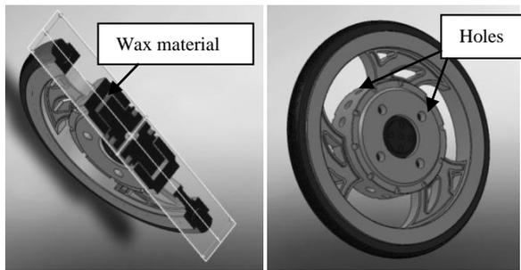
Fig. 2. New design of the scooter wheel (DFAdT analysis)
