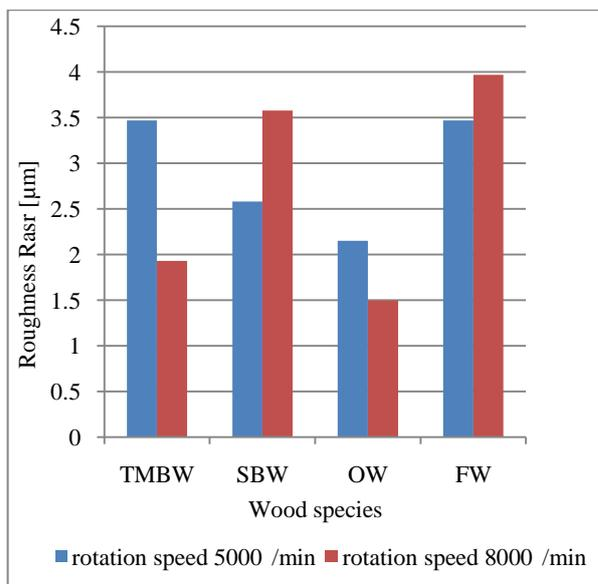
Fig. 2. Comparison of values of roughness parameter  $R_a$  for different rotational speeds (TMBW – Thermally modified beech-wood; SBW – Steamed beech-wood; OW – oak-wood; FW – Fir-wood)
