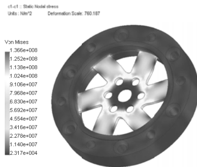
Fig. 2. Equivalent (von Mises) stress of the membranes unit without deviations
