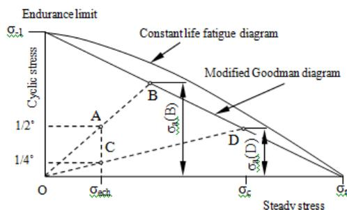
Fig. 3. Modified Goodman diagram for membrane assembly  $\sigma_r$  – ultimate stress;  $\sigma_c$  – yield stress;  $\sigma_{ech}$  – equivalent stress;  $\sigma_{e1}$  – endurance limit
