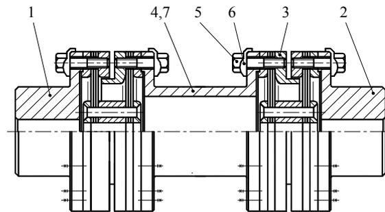
Fig. 1. Spacer coupling (1, 2 – flanged hub; 3 - membrane unit; 4, 7 - spacer; 5 - bolt; 6 – washer)
