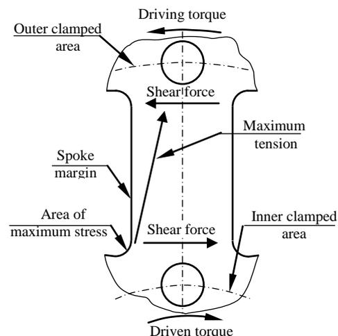
Fig. 2. Loading scheme of an individual membrane spoke
