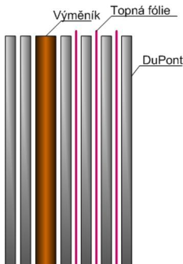
Fig. 3. The section of the thermal panel
