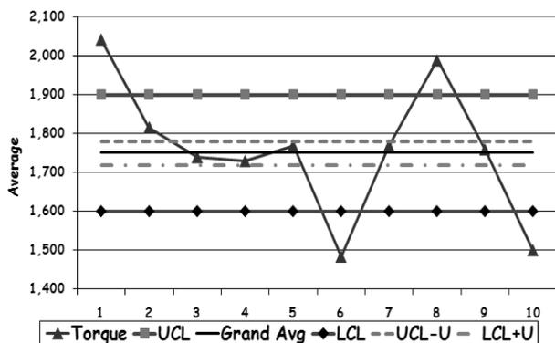
Fig. 2. SPC analysis for the pneumatic screwdriver
