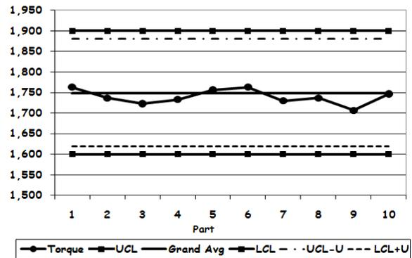
Fig. 3. SPC analysis for the electric screwdriver
