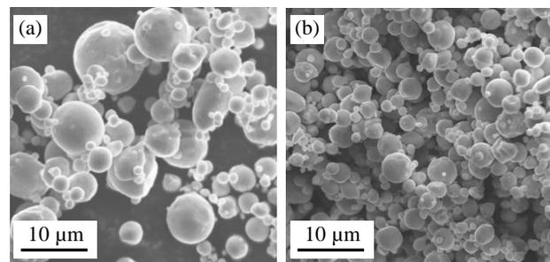
Fig. 1. The SEM micrographs of SS grade 904L –16 μm (a) and –7 μm (b) powders
