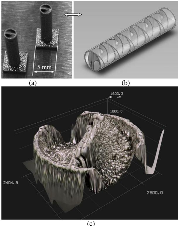
Fig. 3. Mixing element Kenics from SS grade 904L ( $\sim 7 \mu\text{m}$ ) powder: diameter is 3 mm and height is 15 mm (a), internal structure (b), top view (c)
