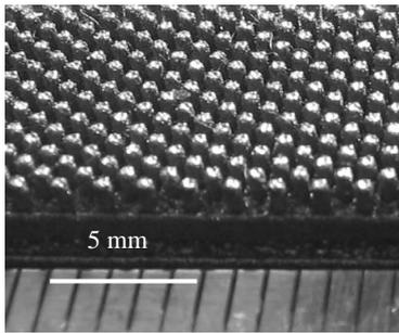
Fig. 2. Sample from SS grade 904L ( $\sim 16 \mu\text{m}$ ) powder with developed structure. The number of pins per unit area is  $175 \text{ pins}/\text{cm}^2$
