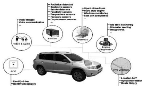
Fig. 3. Sensor network with Open Enterprise AVL Unit
