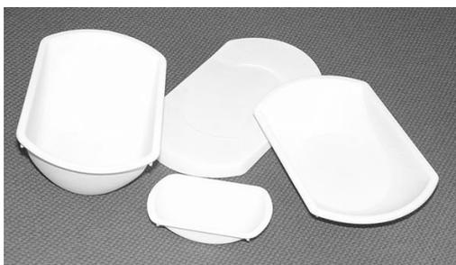
Fig. 5. Margarine containers (SLS prototypes)
