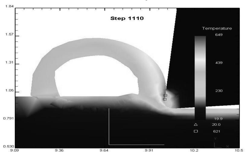
Fig. 1. Temperatures distribution for cutting speeds of de 400 m/min after 0.00152 seconds of simulation
