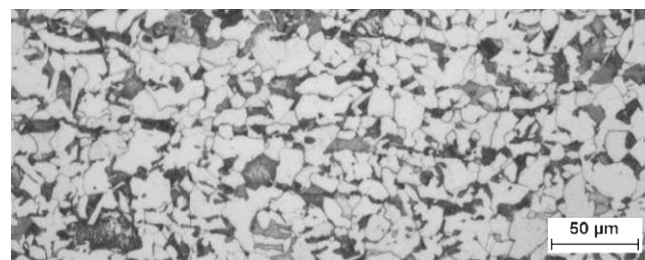
Fig. 2. Steel A, basic model treatment on simulator, Nital
