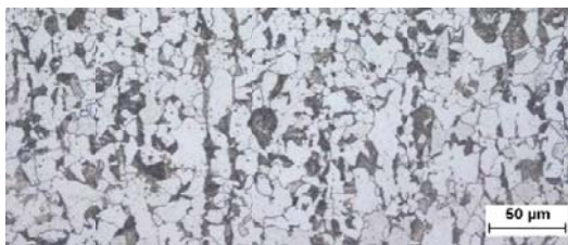
Fig. 4. Steel B, longitudinal section, model with unidirectional 10 mm tension deformation, Nital
