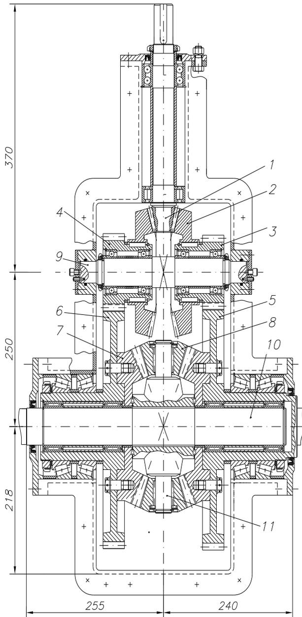
Fig. 1. Cross section on differential gearbox
