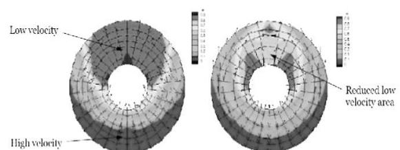
Fig. 2. Wake for initial stern and modified one
