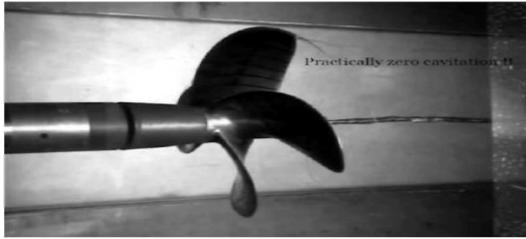
Fig. 3. Simulated nominal wake in the cavitation tunnel
