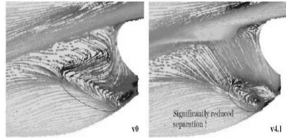
Fig. 5. Limit streamlines on stern surface
