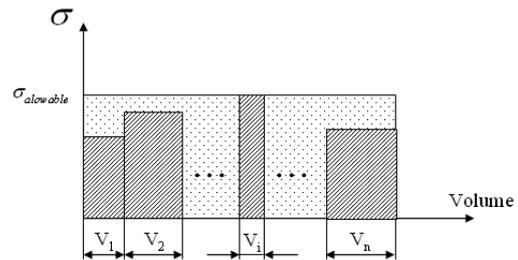
Fig. 1. Structural efficiency for stress on elements criteria
