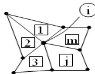
Fig. 2. Node connectivity of elements
