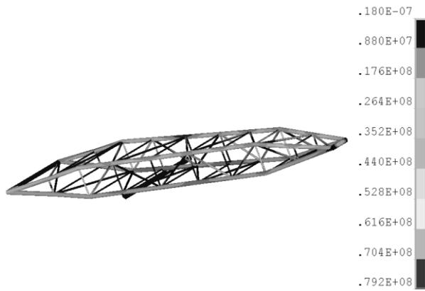
Fig. 3. Stress on elements before optimization
