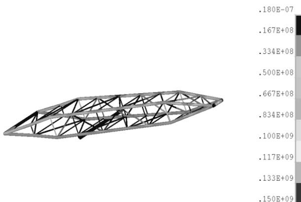
Fig. 4. Stress on elements after optimization
