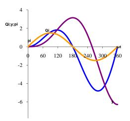
Fig. 1. The diagrams of the pressure, sonic flow and of the racing for the sonic hammer
