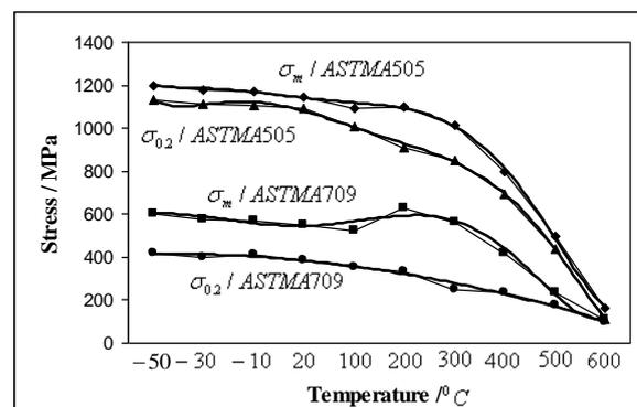
Fig. 1. The effect of temperature (lowered and elevated) on mechanical properties
