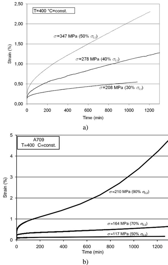
Fig. 2. Creep behavior of ASTM A505 steel and ASTM A709 steel at temperature of 400°C. a) Steel ASTM A505. b) Steel ASTM A709
