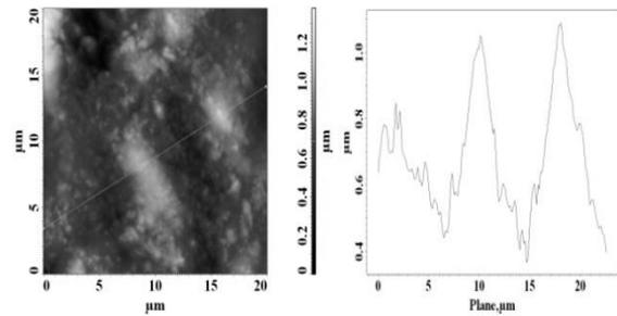
Fig.5. Image and 2D profile of Vertex Soft sample for 20 μm
