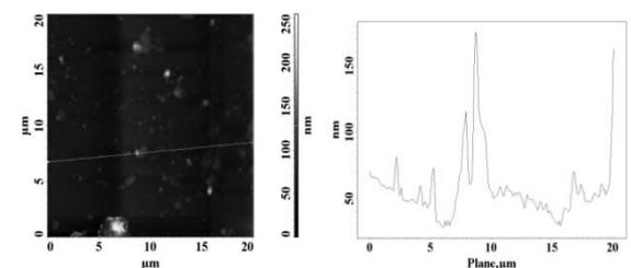
Fig.4. Image and 2D profile of glazed Duracryl Plus sample for 20 μm
