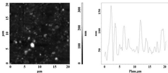
Fig.3. Image and 2D profile of unglazed Duracryl Plus sample for 20 μm
