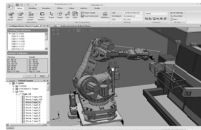
Fig. 4. Setting the robot configuration for the first target of a path
