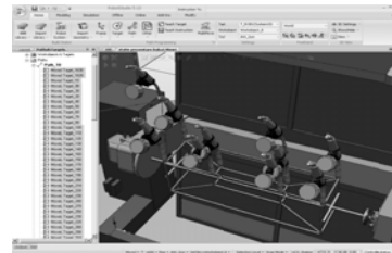
Fig. 3. Setting the tool orientations for each target of a path
