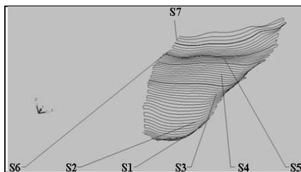
Fig. 3. The graphic results after scanning using the coordinate measuring machine, *DEA GLOBAL Performance*
