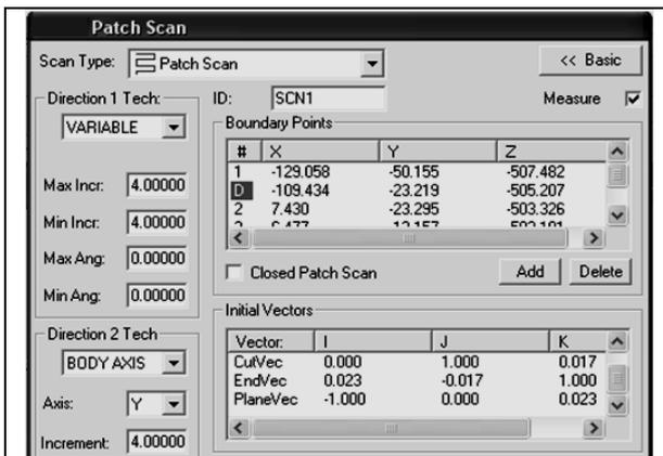
Fig. 2. Definition of scanning parameters for the mould model
