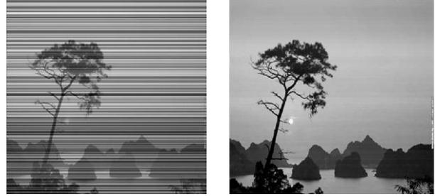
Fig. 2. Result of reading initial image by photo sensor array ( $\delta=98$ ) and result of correction using 3 initial images ( $\delta=5$ )
