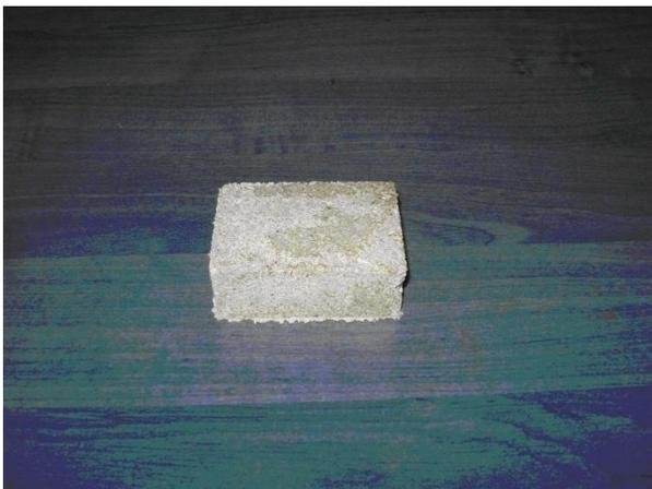
Fig. 4. Silicone rubber obtained from used rubber recycling
